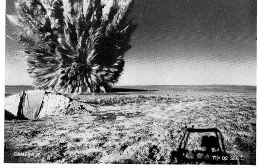
PRE-SCHOONER II blast from 85 tons of liquid nitro-methane starts in this photo. Dotted lines are the cables from the balloon which support blast pressure instrumentation stations. White dots are flags attached at 50-foot intervals along the cables.
